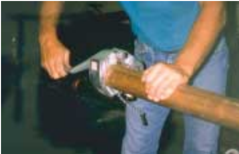
Portable hand roll groovers and power units for 2 - 6" copper; up to 48" steel.
