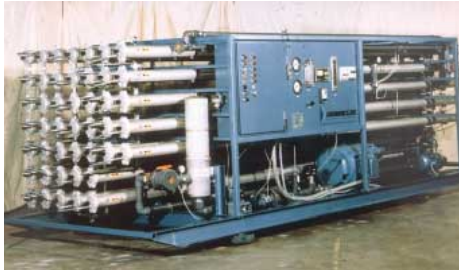
Reverse osmosis grooved end caps allow easy filter membrane cleaning, removal and service.
