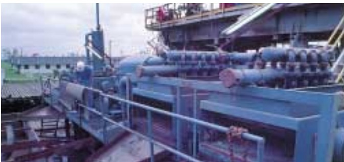
Desanders and desilters utilize Snap-Joint® quick disconnect and standard couplings for easy service.
