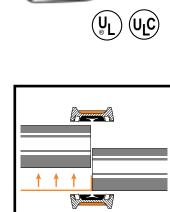
Union at every joint Permits easy access to existing lines • Removal of only two couplings permits removal of pipe, valves or equipment • Permits rotation of pipe
