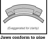
Roust-A-Bout jaws are circumferentially curved to match pipe contour • Provide greater pipe contact for positive grip • Pinned into housing to prevent loss before installation
