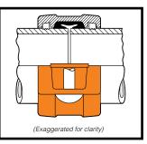
Positive pipe joining Integral grips or jaws provide positive engagement of pipe when torqued to specifications • Suited for pressures up to 750 PSI (5100 kPa) depending upon size
